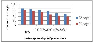
Fig. 9. Durability test in presence of HCL
