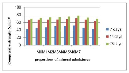
Fig. 1. Overall results of compressive strength
