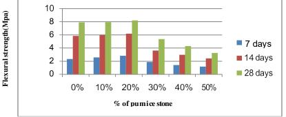
Fig. 6. Graph showing flexural strength of pumice & fibers
