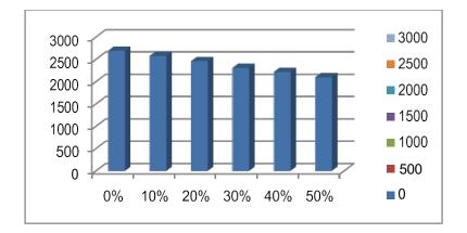
Fig. 7. Density of Light Weight Aggregate Concrete at Different Replacement Levels
